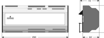
The ECD-000 can be mounted in panels with a 71x29 mm cutout. See dimensional drawing below for space requirements including rear connectors.
