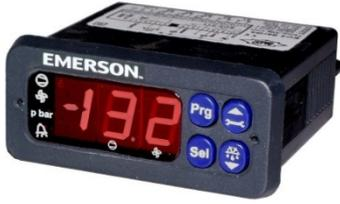
The EC2-552 has been designed to control single compressor or tandem compressor condensing units with a Copeland Scroll Digital™ compressor and variable fan speed control. The purpose of the controller is to maintain suction pressure at a pre-defined level by modulating compressors and to keep condensing pressure to a minimum by varying fan motor speed.
